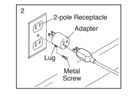
The lug or wire extending from the adapter must be connected with a metal screw to a permanent ground such as a properly grounded outlet box cover. **Some 2-pole receptacle outlet box covers are not** grounded. Before using an adapter, contact a qualified electrician to determine whether the outlet box cover is grounded. The temporary adapter should be used only until a properly grounded outlet can be installed by a qualified electrician.
