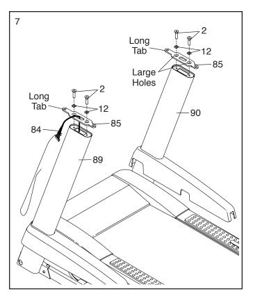
8. With the help of a second person, hold the handrail assembly near the Left Upright (89).
