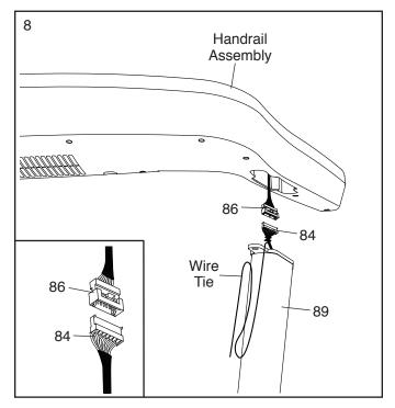
9. Insert the wires into the Left Upright (89) as you set the handrail assembly on the Left and Right Uprights (89, 90). **Be careful not to pinch the wires.**
