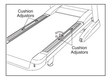
To decrease the firmness, step off the treadmill and use a hex key to turn the cushion adjustors counterclockwise until the number of the desired firmness level appears next to the cushion adjustor (1 is the lowest firmness level).
