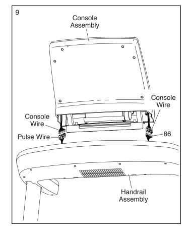
Set the metal bracket on the console assembly on the metal frame inside the handrail assembly.
