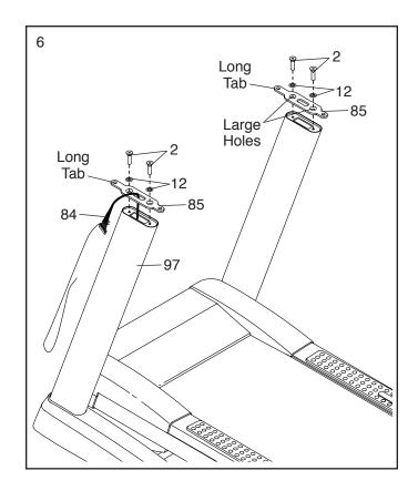
7. With the help of a second person, hold the handrail assembly near the Uprights (97).
