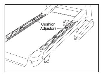
To decrease the firmness, step off the treadmill and use a hex key to turn the cushion adjustors counter-clockwise 1/4 turn until the word "On" appears next to the cushion adjustor.
