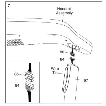
8. Insert the wires into the left Upright (97) as you set the handrail assembly on the Uprights. **Be careful not to pinch the wires.**
