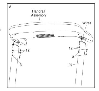
With the help of a second person, hold the console assembly near the handrail assembly. Be careful not to pull on the wires during assembly.
