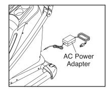
equipped with an AC power adapter having an equipment-grounding conductor and a grounding plug. Plug the AC power adapter into the jack on the front of the elliptical strider. Then, plug the AC power adapter into an appropriate outlet that is properly installed and grounded in accordance with all local codes and ordinances. This product is for use on a nominal 120-volt circuit. IMPORTANT: The elliptical strider is not compatible with GFCI-equipped outlets.
