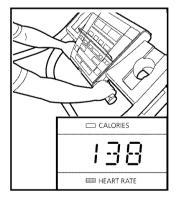
tacts—avoid moving your hands. When your pulse is detected, the Heart Rate indicator will flash and then your heart rate will be shown. For the most accurate heart rate reading, continue to hold the contacts for about 15 seconds.
