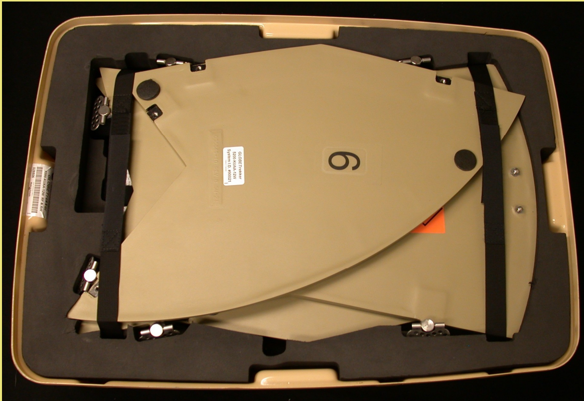
Figure 3 Backpack A - Antenna/RF Lid with Antenna Segments
