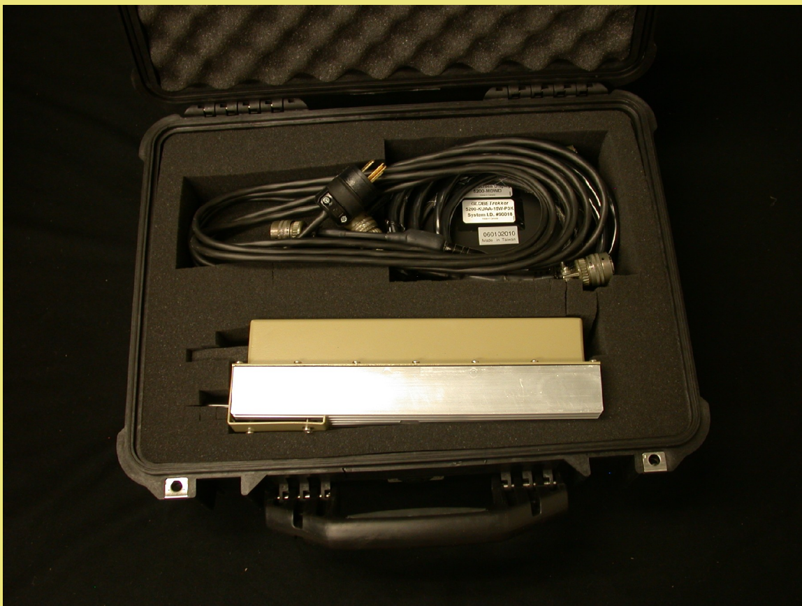
Figure 7 Transit Case C - AC-DC Power Supply
