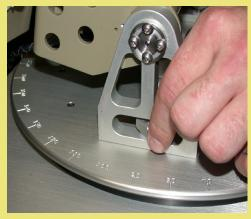
10 Remove the right and left back plate supports of the main antenna assembly from the azimuth plate.
