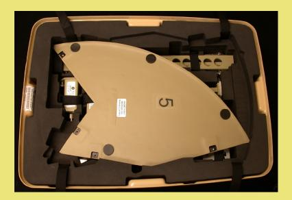
8 Replace antenna segment 4 on top of segment 5 into the top of Antenna/RF backpack (back side facing up).
