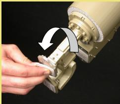
3 Loosen and remove the lower boom arm segment from the main antenna assembly.
