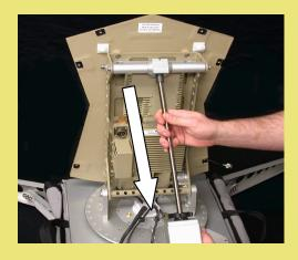
9 Unfasten the left and right back plate supports of the main antenna unit using the thumb screws.
