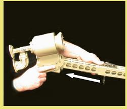
2 Replace protective plastic caps to the feed assembly. Rotate the polarization so that it is pointing directly down.
