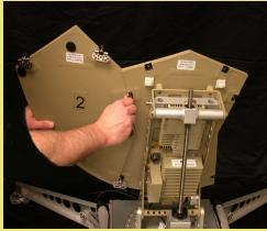
7 Unfasten the elevation assembly unit with the thumb screws.
