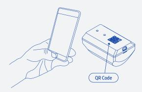
5. Remove the QR code from the back of the detector and attach it to this guide for future reference.
