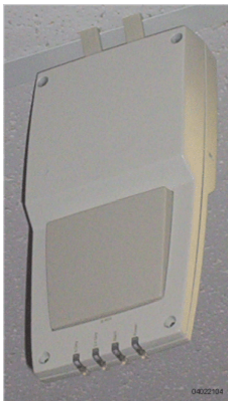
Figure - Clipping the Nortel Networks WLAN - Access Point and Ceiling-Mount Clips to a Hanging-Ceiling Rail
