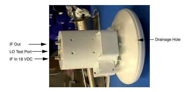
Figure 1-8 CTR 2400 Side View with Brackets
