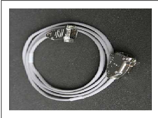
Figure 61 MGC DECT Clock Reference Cable
