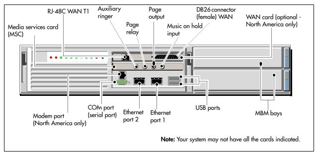
Figure 2 BCM400 main unit ports and connectors
