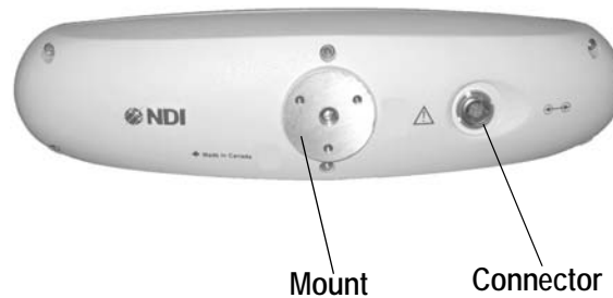
Figure 1-4 Position Sensor - Rear View
