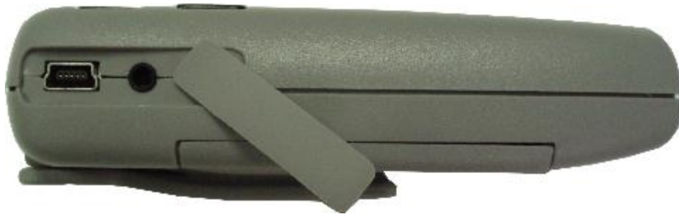
Figure: 4 - Mini MT Side View (Showing USB Port)
