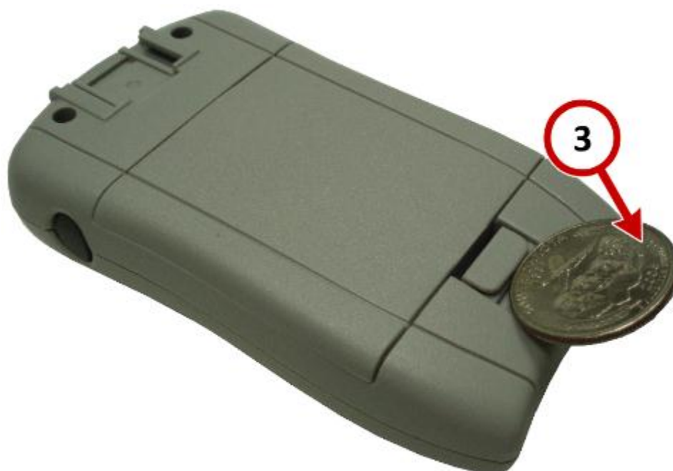
Figure: 7 - Opening the Mini MT battery door.
