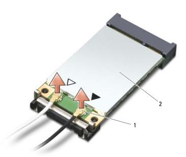
1 antenna cable connectors (2) 2 WLAN card
