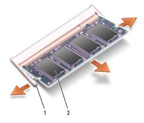
1 securing clips (2 per connector) 2 memory module (DIMM A)
