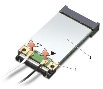
1 antenna cable connectors (2) 2 Mobile Broadband card
