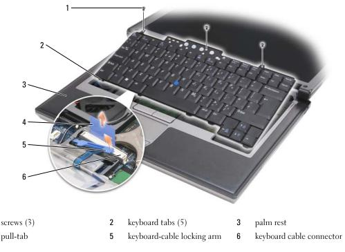
NOTICE: The keycaps on the keyboard are fragile, easily dislodged, and time-consuming to replace. Be careful when removing and handling the keyboard.
