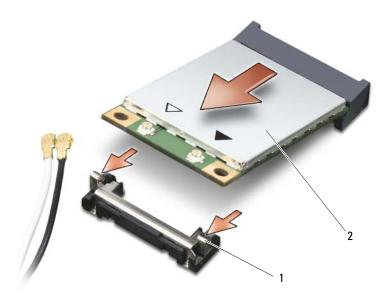
1 metal securing tabs (2) 2 WLAN card
