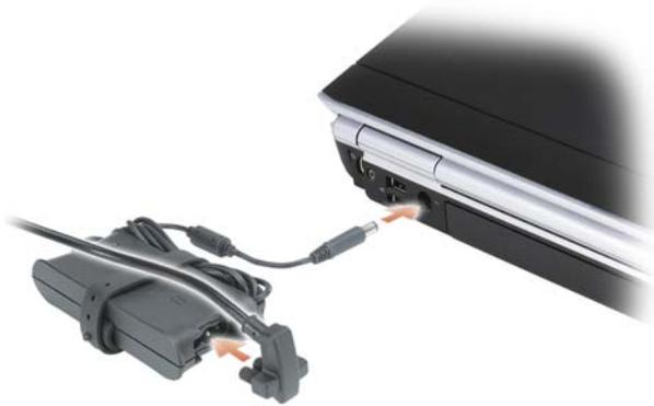
**⚠ CAUTION:** The AC adapter works with electrical outlets worldwide. However, power connectors and power strips vary among countries. Using an incompatible cable or improperly connecting the cable to the power strip or electrical outlet may cause fire or equipment damage.
