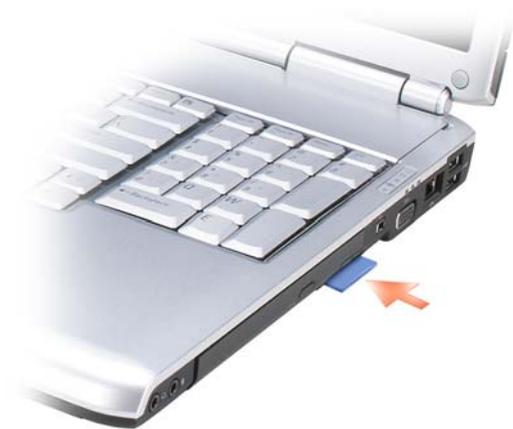
The computer recognizes the memory card and automatically loads the appropriate device driver. If the configuration program tells you to load the manufacturer's drivers, use the media that came with the memory card, if applicable.
