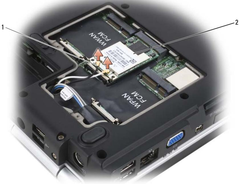
1 antenna cable connectors (2)      2 WLAN card
