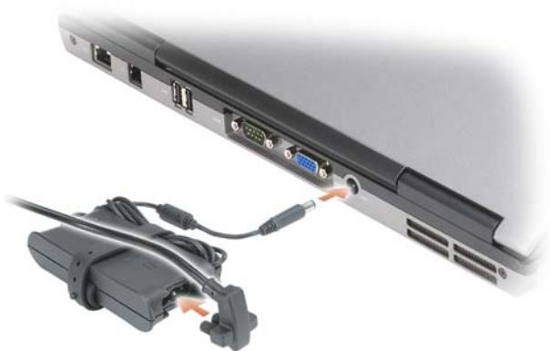
The AC adapter converts AC power to the DC power required by the computer. You can connect the AC adapter with your computer turned either on or off.
