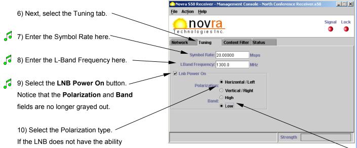
11) If a Universal / Dual LNB is to be used, the Band (Local Oscillator) can be selected here. But in most
