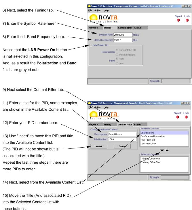
16) Set all of these inputs into the S75 Receiver by selecting "Action" then "Apply" from the drop down menu. **If** any values have been left out or entered incorrectly, the S75 will provide an error message and automatically move to the location of the problem.
