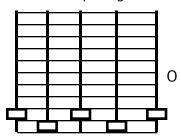
Below is the <u>worst</u> sort of curve to use because you are using EQ to *add volume*. With exaggerated boost you can easily run your power amplifiers into "clipping" and damage your speakers.
