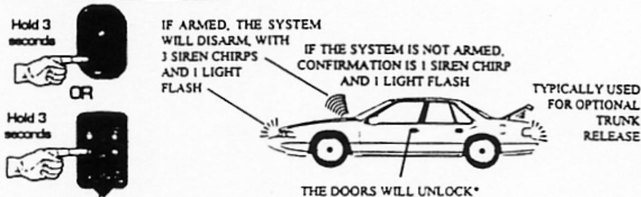
**Press & Hold for 3 Seconds the "Auxiliary Output" Button (II)**
