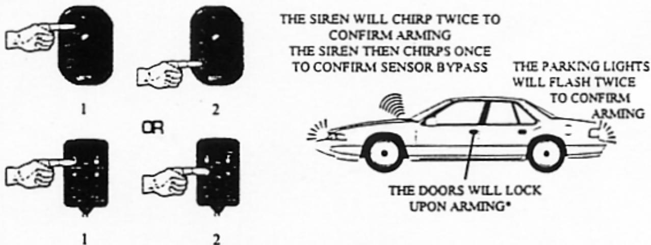
**Press & Release the "Arm/Lock" Button ( ) to Arm, then Press & Release the "Auxiliary Output" Button (II)**
