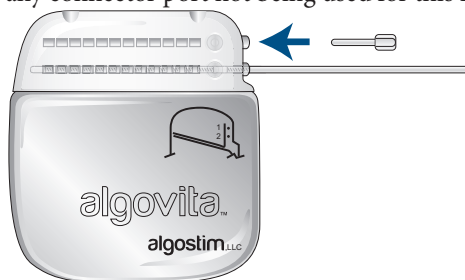
Figure 9. Insert a port plug into any unused port.
