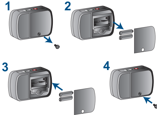
Figure 8. Replacing the EPG batteries
