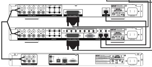
Once these connections are complete, the Control Pads can be addressed for a twelve-zone system.
