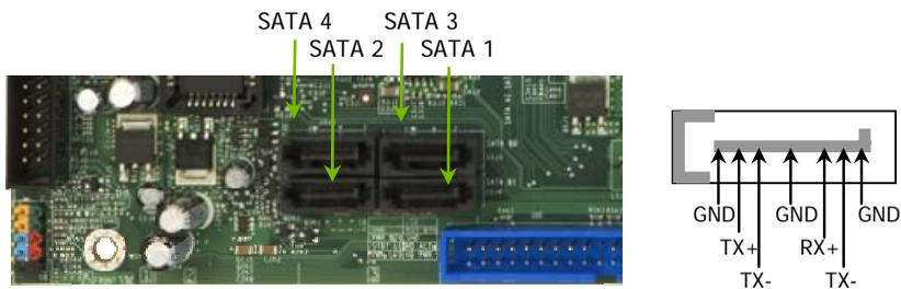
1. Connect the locking cable end to the motherboard connector.
