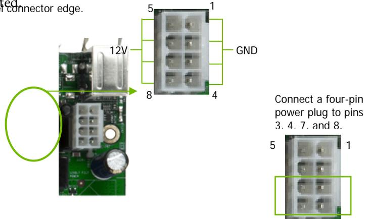
It is *strongly* recommended that you use an 8-pin ATX 12V power supply; however, if you have a four-pin power supply, plug the connector to pins 3, 4, 7, and 8 as shown.
