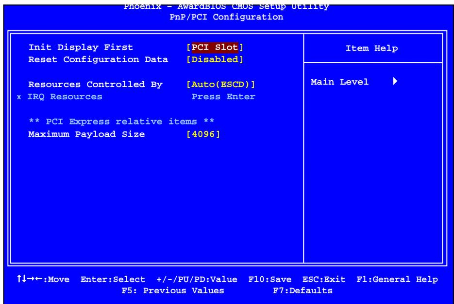
Figure 15. PnP/PCI Configuration Menu
