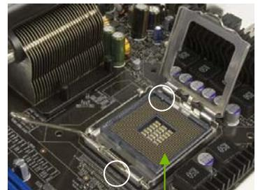
Align notches with notches on the CPU
