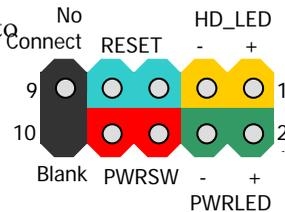
**Note:** The power LED cable in some chassis is a three pin connector with the pins installed in positions 1 and 3. If your chassis has a three pin connector, you will need to remove pin 3 and put it into position 2 or you can use a pair of scissors to cut out position 2. Most chassis come with a two pin connector.
