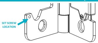
If the Door Hinge Sensor does not update its status as "Closed" when you close your door, then your door may not have good alignment. You will need to install one of the supplied set screws at the location shown above, opposite the Contact Lever.
