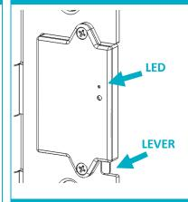
Test the Sensor from desired location before installation. Push and release the Contact Lever gently and insure that the icon on your web portal or smart phone application updates with a "Closed" and "Open" status. Installation on metal can reduce transmission range. Ensure that the device is installed in a dry location away from water, moisture, and rain.
