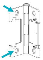
Mount the Door Hinge Sensor to the door edge, insuring that it is properly seated in the door edge recess. You may need to apply pressure to your door to bring it into alignment. You may use the screws removed from the existing door hinge.
