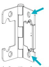
Mount the Door Hinge Sensor to the door frame, insuring that it is properly seated in the door frame recess. You may use the screws removed from the existing door hinge.
