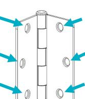
For best aesthetics, install the Door Hinge Sensor in the lowest door hinge position.
