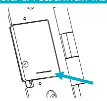
Pull the plastic tab from the backside slot in the Door Hinge Sensor's wireless module. The LED Power Up sequence should be visible on the front-side of the wireless module.
