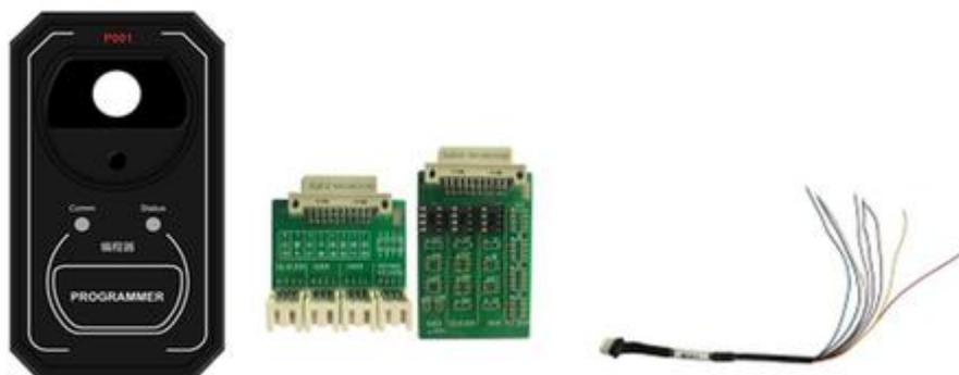
Note: Not all configurations include P001 Programmer accessories. P001 Programmer is used for key transponder renewing and EEPROM reading and writing functions, the wiring of key renewing (specific function operation is helpful in software) is as shown below.
