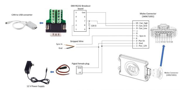
The Can\_High, Can\_low & Can\_Gnd are differential signals and it should be twisted among themselves only. These wires should not be twisted with other wires. This way we reduce interference between signals.
