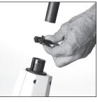
1. Release seat clamp and remove seat and post.
