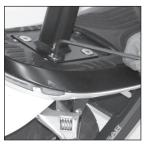
4. Remove four Allen head bolts and lock nuts (tools not included). To perform this operation you will need a six millimeter Allen wrench and a 17 millimeter open end or crescent wrench.
