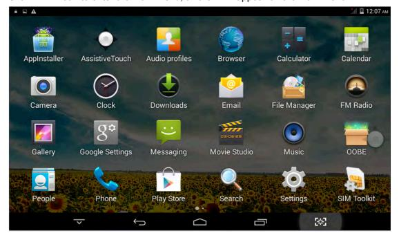
On the main menu, the third-party applications (user-installed applications) can be unloaded. Specific unloading operations are: long press APK want to uninstall, drag it to the top of the desktop, the desktop will appear above the "Uninstall" words, then drag the icon there, you can uninstall the corresponding application as shown below:
