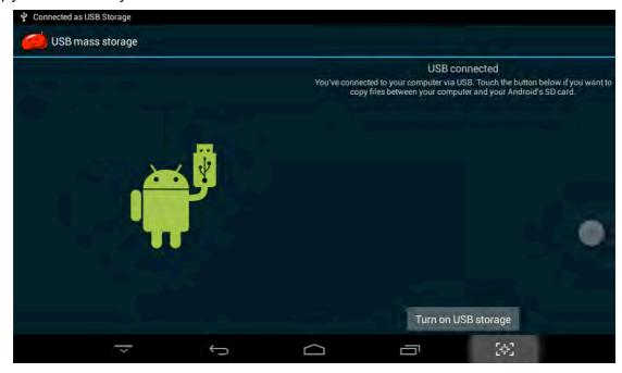
Touch "Turn off USB storage" and then safely remove your device from the computer to prevent data loss.
