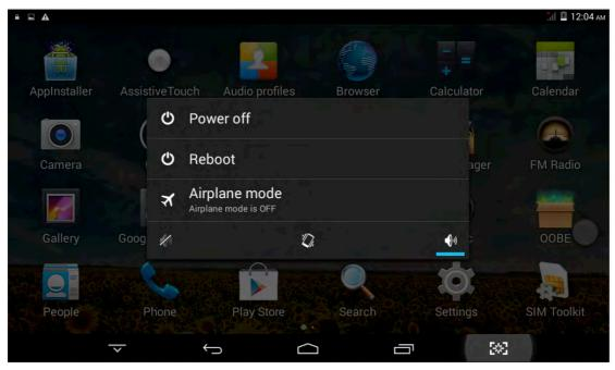
**Standby:** During the power on mode, press the power button to enter the power-saving standby mode, then press the power button again, the screen prompts to enter the unlock mode.
