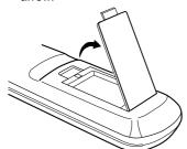
2 Install two "AA" batteries (supplied), paying attention to the polarity diagram in the battery compartment.
