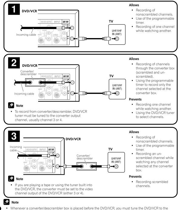
output of the converter/descrambler box, usually channel 3 or 4.
