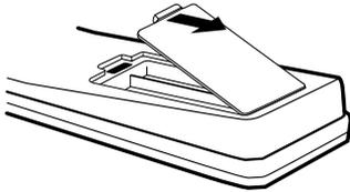
**2** Install two "AAA" batteries (not supplied), paying attention to the polarity diagram in the battery compartment.
