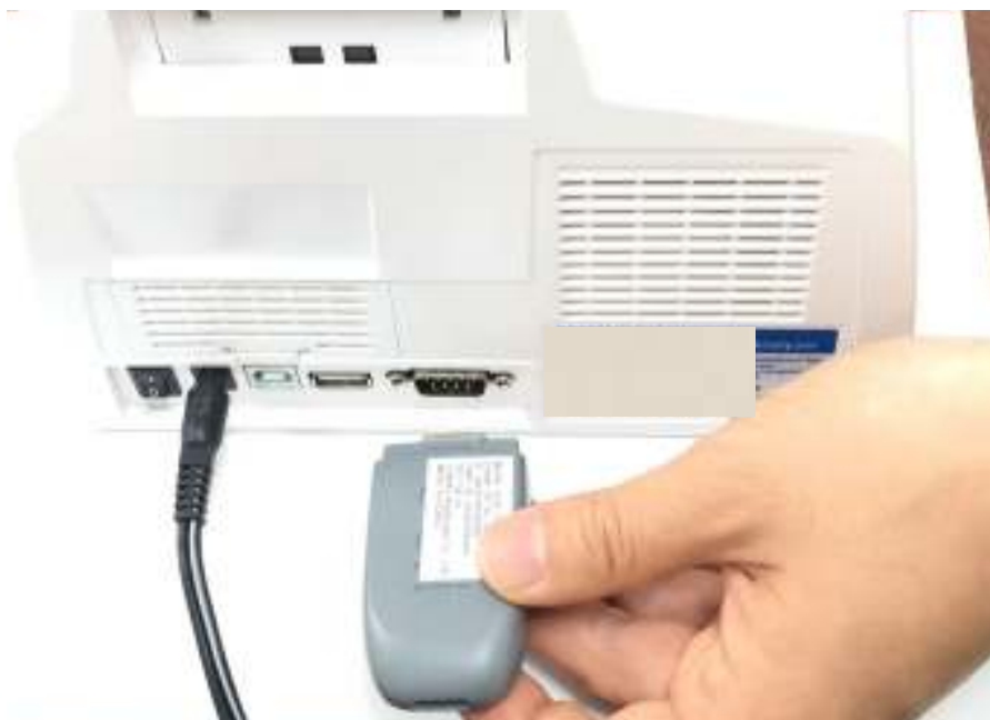
Figure 7 . Oh'Care Bridge on D-Sub 9
