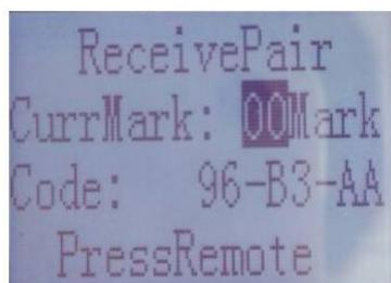
XX-XX-XX: Showing transmitter codes. No codes means no pairings.
