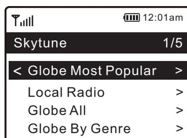
Note - You can change the Local Radio area under **Configuration > Local radio setup**. Please refer to section 10 for the details.
