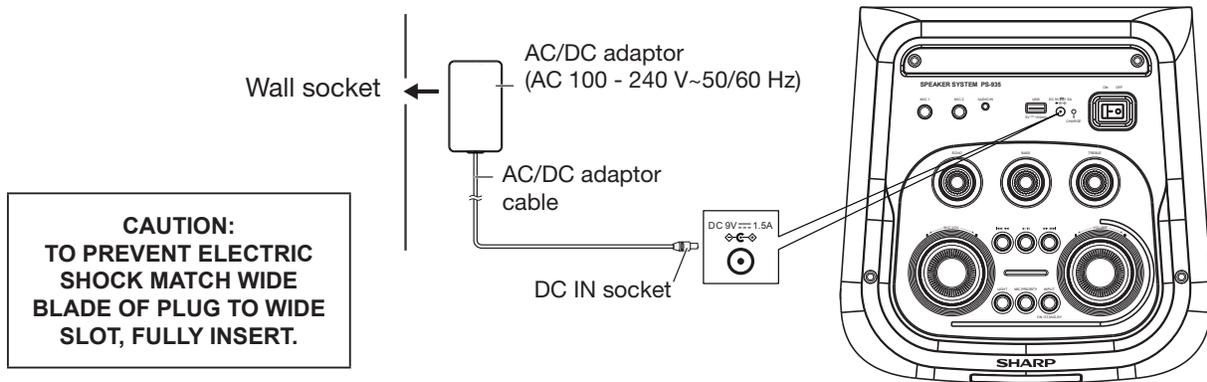
Before using this unit, it is recommended that the internal lithium-ion battery is fully charged. When fully charged, remove the AC/DC power adaptor from the AC socket. When the battery charge is low, the charge light will flash red.
