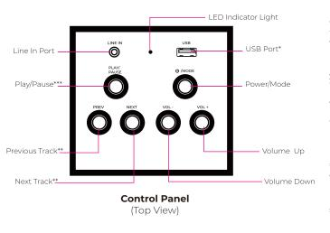
\*You can insert most thumb drives or jump drives into the USB Port. Your speaker can play. MP3, or. WAV music files stored on your drive. Note that the USB port cannot be used to charge your electronic devices.
