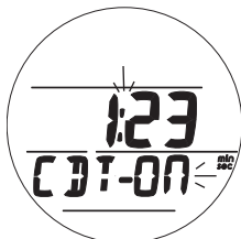
Fig. 112 - CDT STATUS (On, running)
