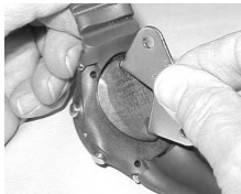
Fig. 132A - COVER REMOVAL (using tool)
