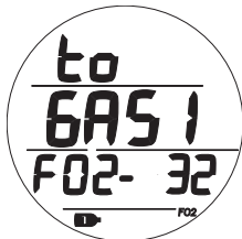
Fig. 98 - GAS 1 SWITCH PREVIEW
