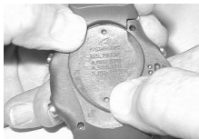
Fig. 132B - COVER REMOVAL (using thumbs)
