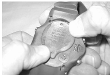
Fig. 136B - COVER INSTALL (using thumbs)
