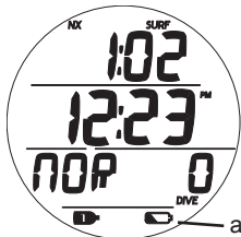
Fig. 1 - SURFACE MAIN (low battery warning)
