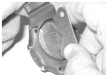
Fig. 136A - COVER INSTALL (using tool)
