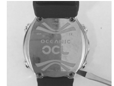
Fig. 134 - TO LOOSEN BATTERY COVER
