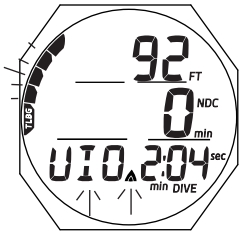
Fig. 127 - VIOLATION (Deco entry, during audible)
