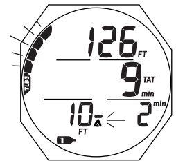
Fig. 74 - DECO ENTRY (during audible)
