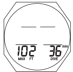
Fig. 99B - GAUG DIVE ALT 1 (if Timer is on Main)
