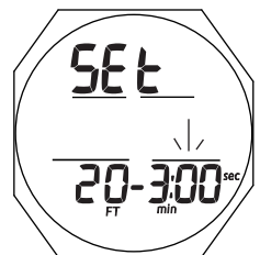
Fig. 50 - SET SAFETY STOP (Time then Depth)
