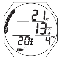
Fig. 75 - DECO STOP MAIN
