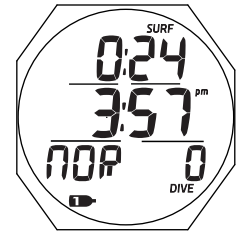
Fig. 24A - NORM SURF MAIN (no dive yet)
