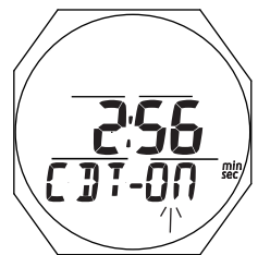
Fig. 106A - CDT STATUS (On, running)
