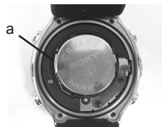
Fig. 136 - RELEASE BATTERY TERMINAL
