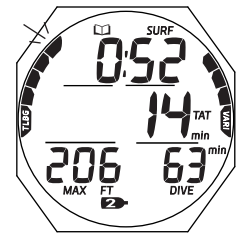
Fig. 33B - LOG DATA 1 (Deco during dive)
