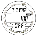
Fig. 108 - FREE CDT STATUS (OFF/READY)
