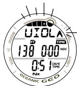
Fig. 86 - VIOLATION GAUGE MAIN
