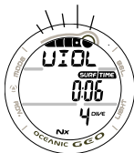
Fig. 87 - VIOLATION GAUGE SURFACE
