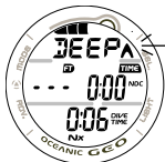
Fig. 85 - DELAYED VIOLATION #3 MAIN
