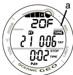
Fig. 78 - DECO STOP MAIN
