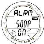
Fig. 21 - DAILY ALARM STATUS
