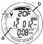
Fig. 82 - CONDITIONAL VIOLATION MAIN
