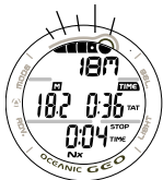
Fig. 84 - DELAYED VIOLATION #2 MAIN
