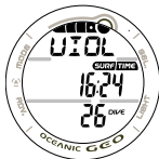
Fig. 115 - FREE SURF VIOLATION (DECO)
