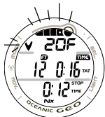
Fig. 83 - DELAYED VIOLATION #1 MAIN
