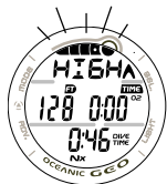
Fig. 25 - O2 EX- CEEDED
