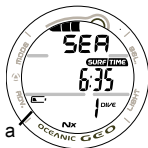
Fig. 3 - LOW BATTERY WARNING
