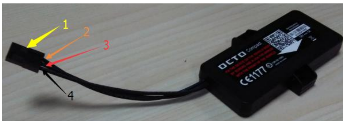
Figure 3. Power Supply Terminals
