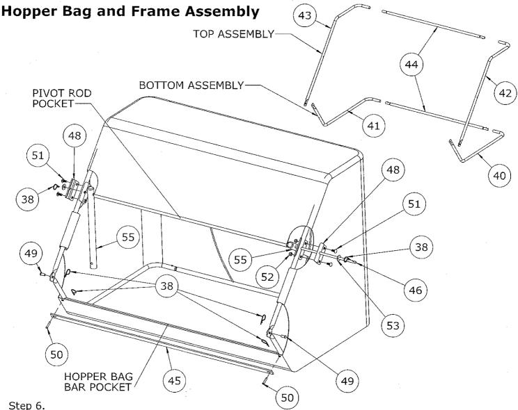
Build bottom assembly. Connect bottom left tube (40), center tube (44), and bottom right tube (41). Slide hopper bag bar (45) into the pocket provided on front bottom of the bag. Insert bottom assembly into hopper bag. Connect the bag, bar and tubes by inserting clevis pins (50) thru grommet on bag, bag bar, and tube. Lock it in place with hairpin cotter (38). Repeat for other side.
