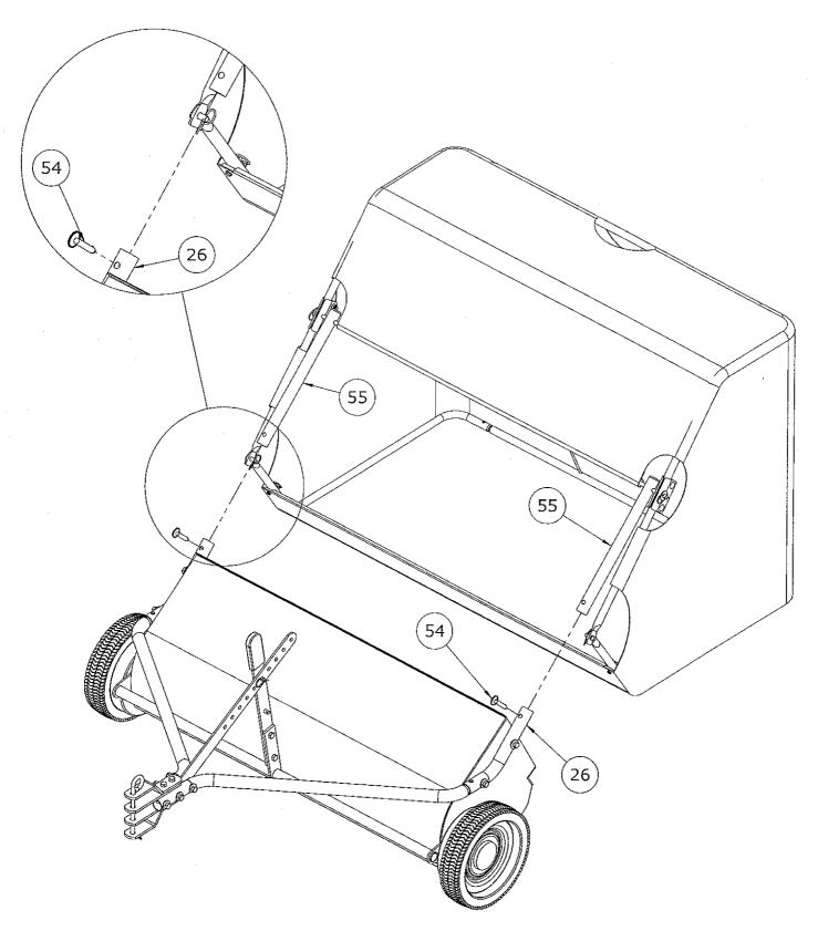
Step 10. Insert hopper connect tubes (55) into hitch mount tubes (26) as shown and lock in place with 3/8" ring grip pins (54).
