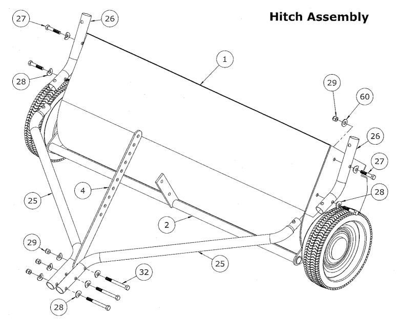
NOTE: MAKE SURE HEIGHT ADJUSTMENT PLATE (4) IS ABOVE HEIGHT ADJUSTMENT TUBE (2) WHEN ASSEMBLING.
