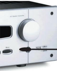
3. Self-adhesive "Flashers" affix to the Infrared sensors on the front panels of your components. The Flashers relay commands to components out of sight of the MRZ-260 Front Blaster. The flashers plug in to the MRZ-260 rear flasher line outputs via their 10 foot cables. Uniquely, the MRZ-260 can also connect to components with rear panel IR Inputs via its adjustable IR Line Outputs.
