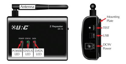
Power LED: Indicates that the ZR-1N is powered on when illuminated.
