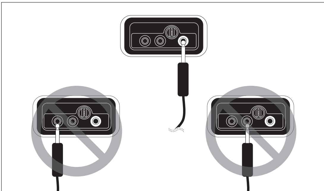
Figure 6.1 CAUTION - Correct connection of a monopolar 1-pin plug with a 4 mm pin diameter
