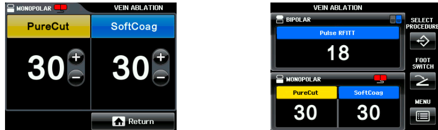
Figure 7.5 Split type indicator for CQM shining red on the Set Screen and on the All Screen
