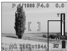
The cursor moves up and down on the zoom indicator according to the zoom magnification. The cursor turns orange when inside the digital zoom field.
