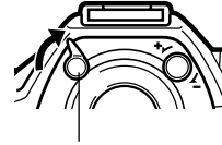
Eyepiece shutter lever
