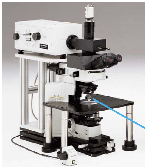
BX61WI fixed stage upright microscope+translation stage
