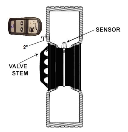
For dual-wheel assemblies, position the SmartWave LF Tool approximately 2 inches (5 cm) away from the tire's surface positioned at the center of the outboard tire's sidewall opposite the valve stem. The transmission from the tool will pass through the outboard tire and provoke a data transmission from the sensor mounted on the inboard tire.
