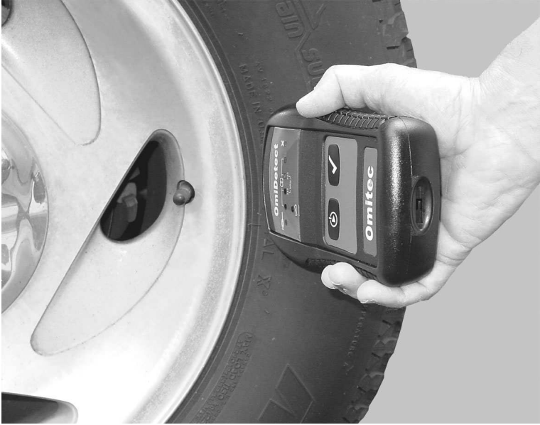
Figure 1. OmiDetect shown in use in testing a TPM sensor.
