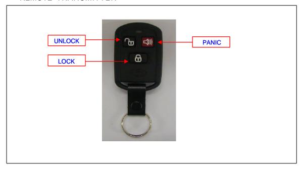
You can lock and unlock your vehicle with the remote transmitter.
