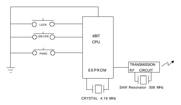
figure 3.1 block diagram of the transmitter
